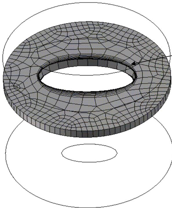
2-D boundary layer on source face is distorted during Cooper projection
