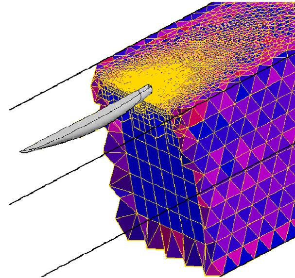
Flow Volume Around a Boat Hull
