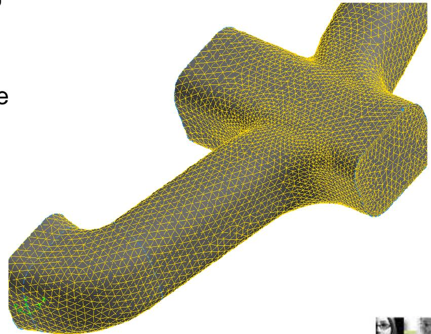
Manifold Geometry with tet-dominant mesh using sizing functions and boundary layers
