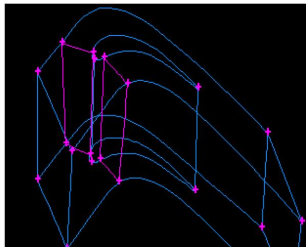
Vertices can be adjusted after meshing (might require subsequent smoothing of mesh)
