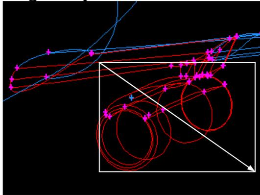
Picking 'completely included' entities when dragging box diagonally up
