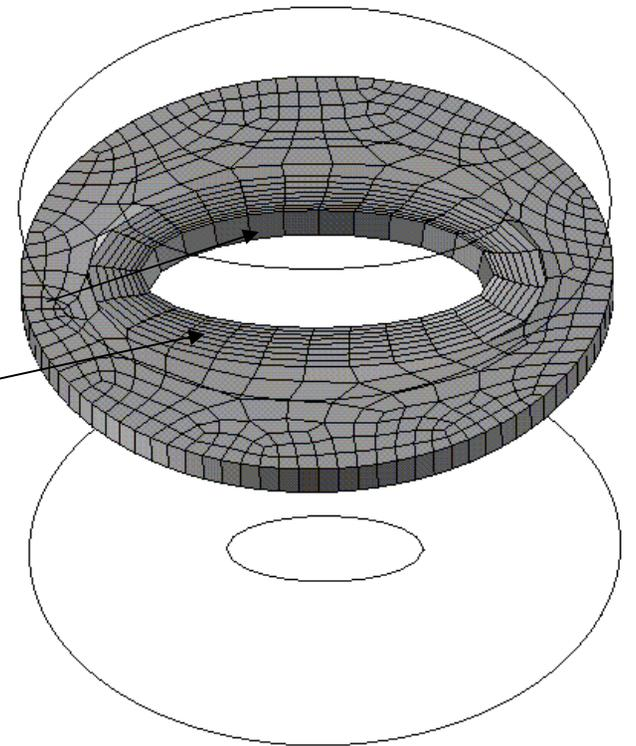
Undistorted "true" cells present due to 3-D boundary layer on side face.
