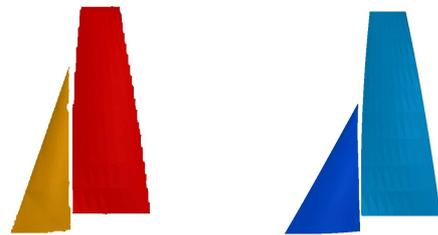
Figure 15 Geometric characteristics of an optimised jib for two different mainsail twist values
