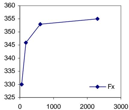
Figure 2: driving force convergence with mesh refinement (number of cells divided by 1000) on GAMBIT mesh and FLUENT solver
