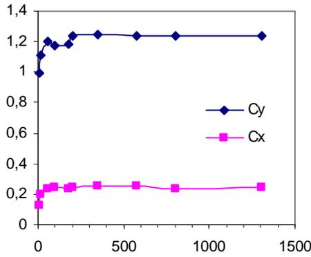
Figure 4 : driving and heeling coefficients convergence (number of cells divided by 1000) with SnappyHexMesh mesh and OpenFOAM solver.
