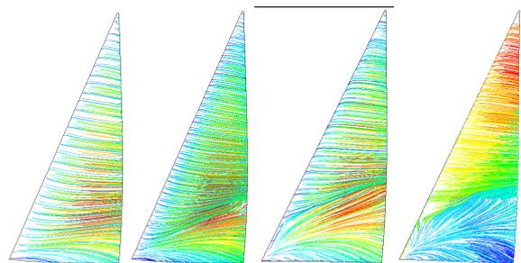
Figure 3 : friction lines on leeward side convergence with mesh: M1, M2, M3, and M4
