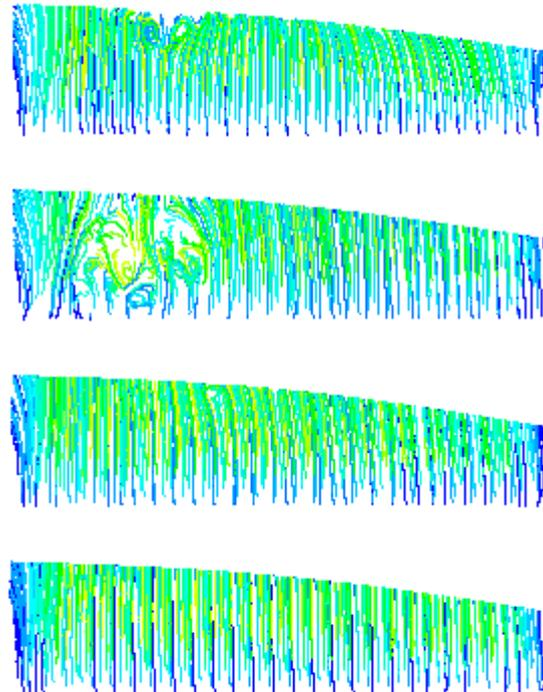
Figure 5 : friction lines on selected sail designs showing convergence toward an optimized design.
