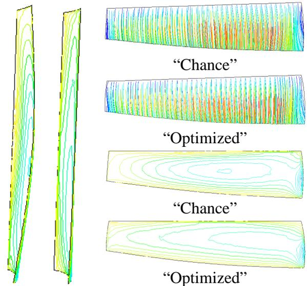
Figure 10 : (left) Chance / Optimized solution with pressure on leeward side (right) friction lines and pressure on leeward side
