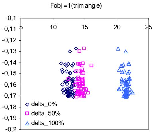
Figure 9 : objective function versus sail trim angle of the three cuts when the heeling moment constraint is satisfied
