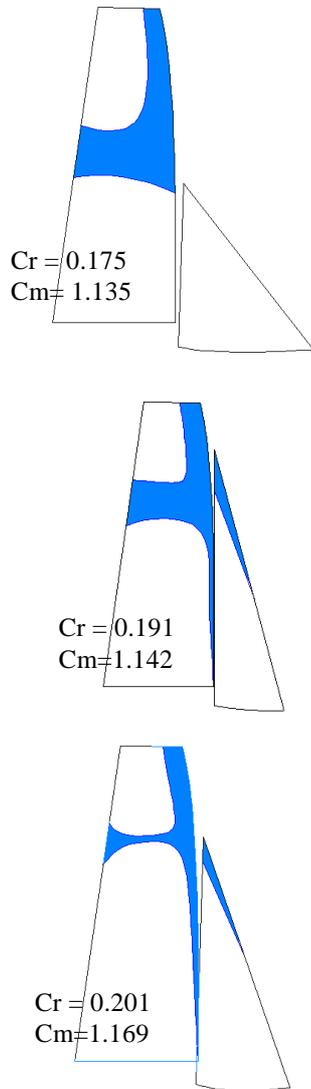
Figure 13 : separated regions on leeward side of the rig for three jibs of different aspect ratio (AR=3.2, 7.9, and 6.1)
