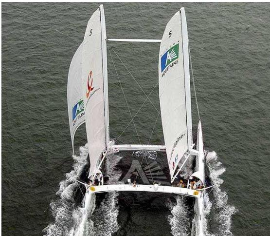
Figure 9: Hydraplaneur double rig
