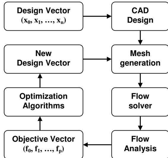
Figure 3: *ADONF* software package diagram
